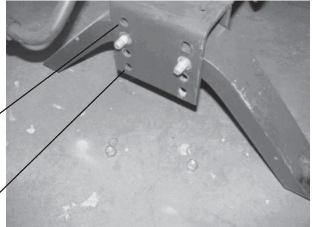
Figure 2-Left Side Frame Mounting Nuts removed
